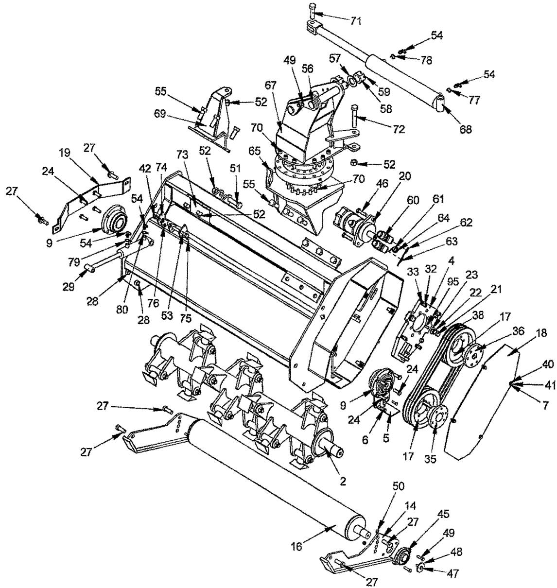
**48 IN FLAIL AXE HEAD ASY - PISTON MOTOR - SWIVEL MT (PART 2)**
